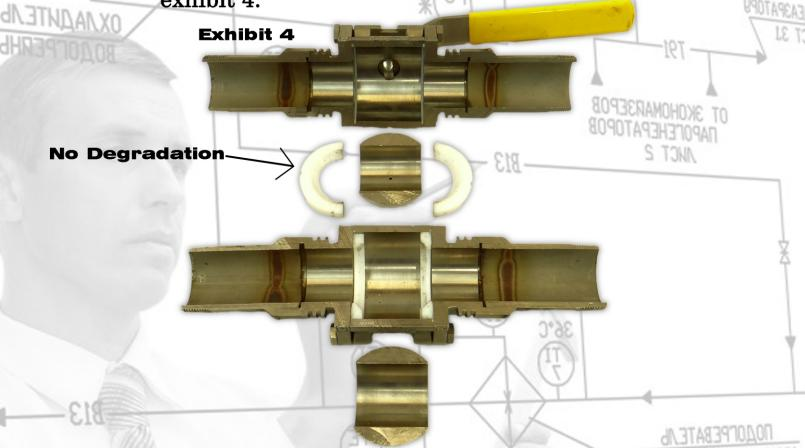
**Test affirmation:** The weld-in-place valve-end heat diffusion technology (see exhibit 1.) dissipated any damaging heat from reaching the seats.
